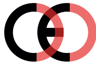
False CE Mark (too close)
