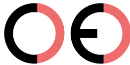
False CE Mark (too far)
